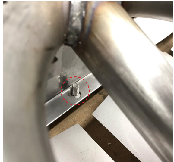
U-burner bracket in proper position on the threaded stud.
