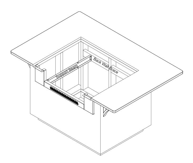
**STEP 3:** Check dimensions of frame construction fit by placing assembled Trim Kit base into prepared cabinet. Mark location for Back Wall Brace. Align Support Beam to marked position of Back Wall Brace and check to ensure Support Beam is level and the Front Panel is positioned to be flush with the front cabinet construction. Attach Support Beam to Back Wall Brace using suitable construction screws (not included).
