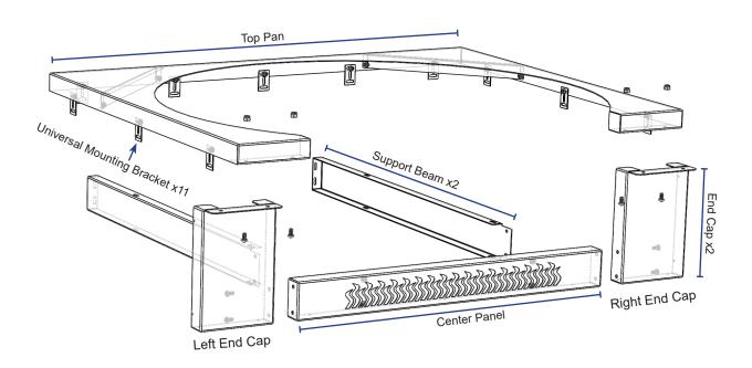
The Trim Kit for the Evo Affinity 25G is shipped partially assembled and requires installation and final assembly. Included in the kit are six (6) separate stainless steel metal components and one (1) package of hardware as listed below:
