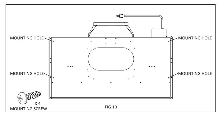
Mounting surface must be a minimum of 3/4" thick. Mount Vent Hood to desired construction using #10 wood screws. A minimum of four #10 wood screws are needed to mount the Vent Hood. Longer screws may be required if wall board or other nonstructural surfaces are used between the hood and the main mounting surface. Anchors may be required if mounting screws do not engage the wood structure.
